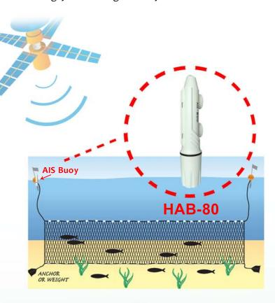
HAB-80 AIS Fishing Net Tracking Buoy unit uses advanced AIS technology to transmit the combined data that include the unique ID and the position of a net. And the data can be received effectively by the vessel equipped with AIS device, then easily recognized and find back the nets with HS-ANT. Also it can avoid collision accidents by other boats.
